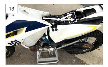
Re-torque all the fasteners after 100 miles.
